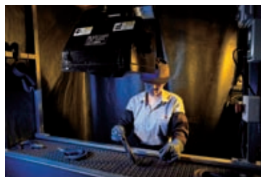
Magnaflux Crack Detection
